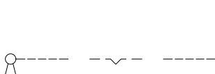
25 keylock switch actuator 3 positions, keylock switch actuator 3 positions for flush mounting page 305, 317
