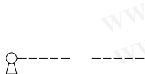
23 keylock switch actuator 2 positions, keylock switch actuator 2 positions for flush mounting page 304, 316
